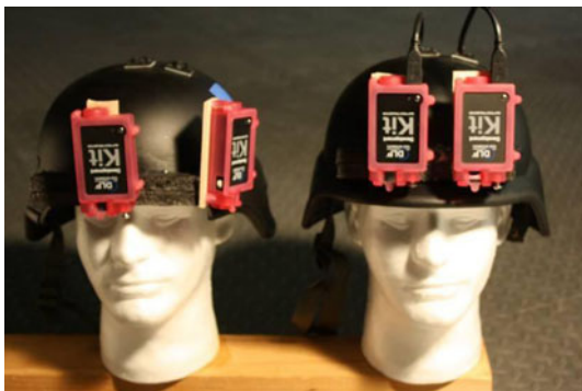
Fig. 5 Experimental projector configurations for a wider field of view ( left ) or for 3D stereoscopic imagery ( right )
