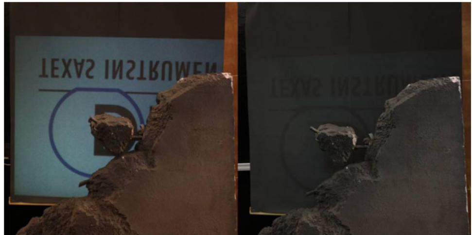
Fig. 3 The retroreflected illumination level near the optical axis of the pico-projector ( left ) is much less than the retroreflected illumination level at 16 inches from the optical axis ( right ). This screen was placed behind a concrete wall prop
