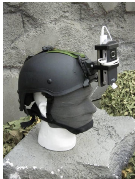
Fig. 6 A prototype REFLCT module, powered by a smartphone, is compact enough to attach to a night vision goggle mount for military training
