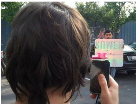
Fig. 4 A test of retroreflective sign material and a projector/mobile phone during daylight. The projection is still very discernable to the user
