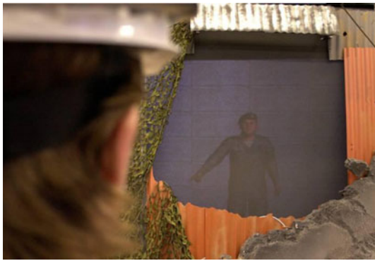
Fig. 2 An over the shoulder view of an animated virtual character, projected on a retroreflective surface by a REFLCT helmet
