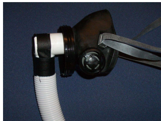
Fig. 2. Prototype breathing mask. This mask attaches to the Spirometer and airflow controller.
