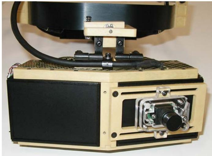
X-travel bridge attaches to Wide5 HMD using two #4-40x0.5 flat head cap screws. Use a 1/16 Allen wrench. Screws thread in to center beam. The process is the same for assembling and mounting the right eye camera.
