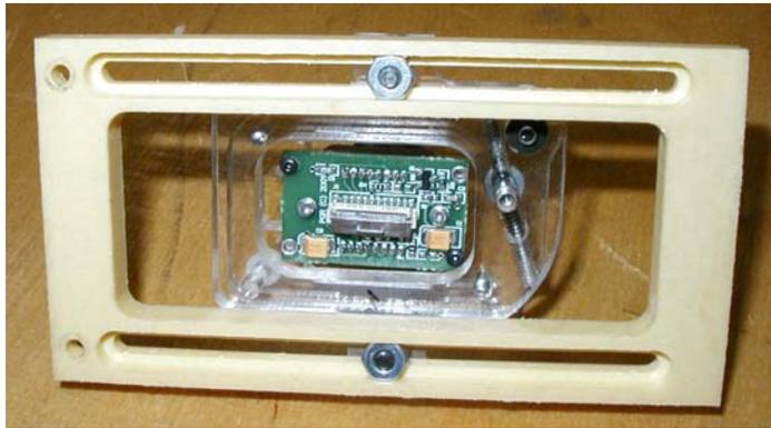
The #4 nuts sit in grooves on the back of the x-travel bridge.
