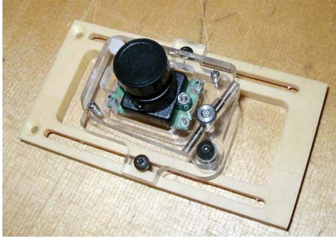
Camera mount attaches to x-travel bridge using two #4-40x0.5 button head cap screws and nuts. Use a 1/16 Allen wrench.
